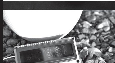
LCD display showing temperature inside the cooker
